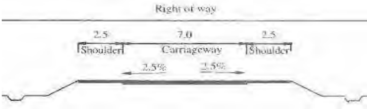
Figure 2.3: TCS. 2.3 Of Schedule D of CA Two lane undivided highway with granular shoulder in Open Country
